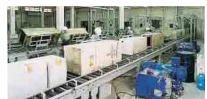
Hirakata Plant refrigerator disassembly line
