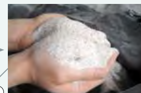
2. Pulverized product Pulverized product is mixed with clay and feldspar (*1) to make material for tiles, then wet ball-milled (*2).
