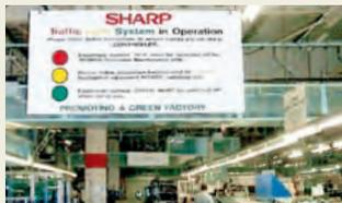
Promoting energy savings by using colors to signal the power-off status of equipment: red means "cannot be turned off except by authorized persons," yellow means "can be turned off when confirmed by authorized person," and green means "can be turned off by anyone."
