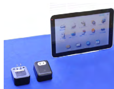
Intelligent power-measuring plugs (left) and media tablet
