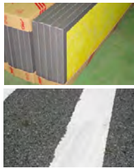
Scrap glass used effectively as an insulation material (top) and in reflective marking materials for lane stripes on roadways
