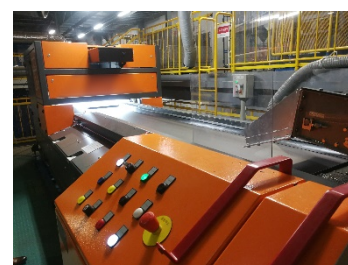
Color sorting machinery for sorting out copper and aluminum
