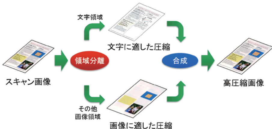
図4 高圧縮PDFの処理概要 Fig. 4 An overview of high compression PDF process.
