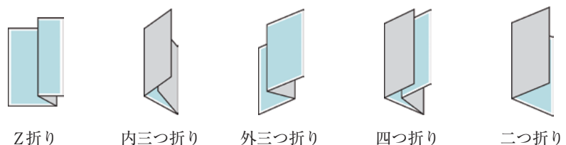
図10 紙折り機での折り方の例 Fig. 10 Example of how to fold in the paper by folding unit.
