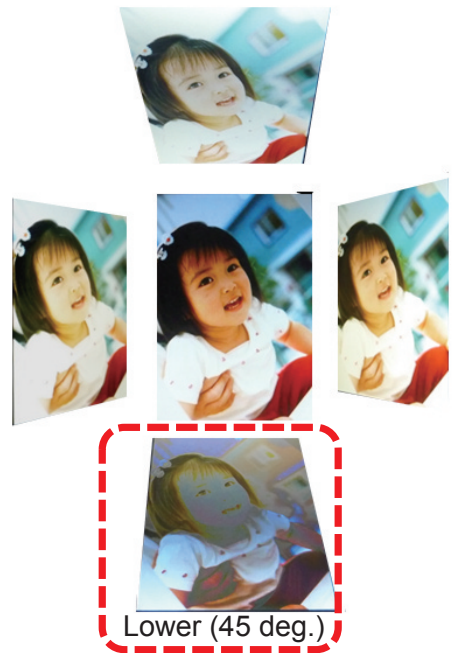
図3 TN液晶の視野角依存性を示す写真 Fig. 3 Photographs of viewing angle dependence.
