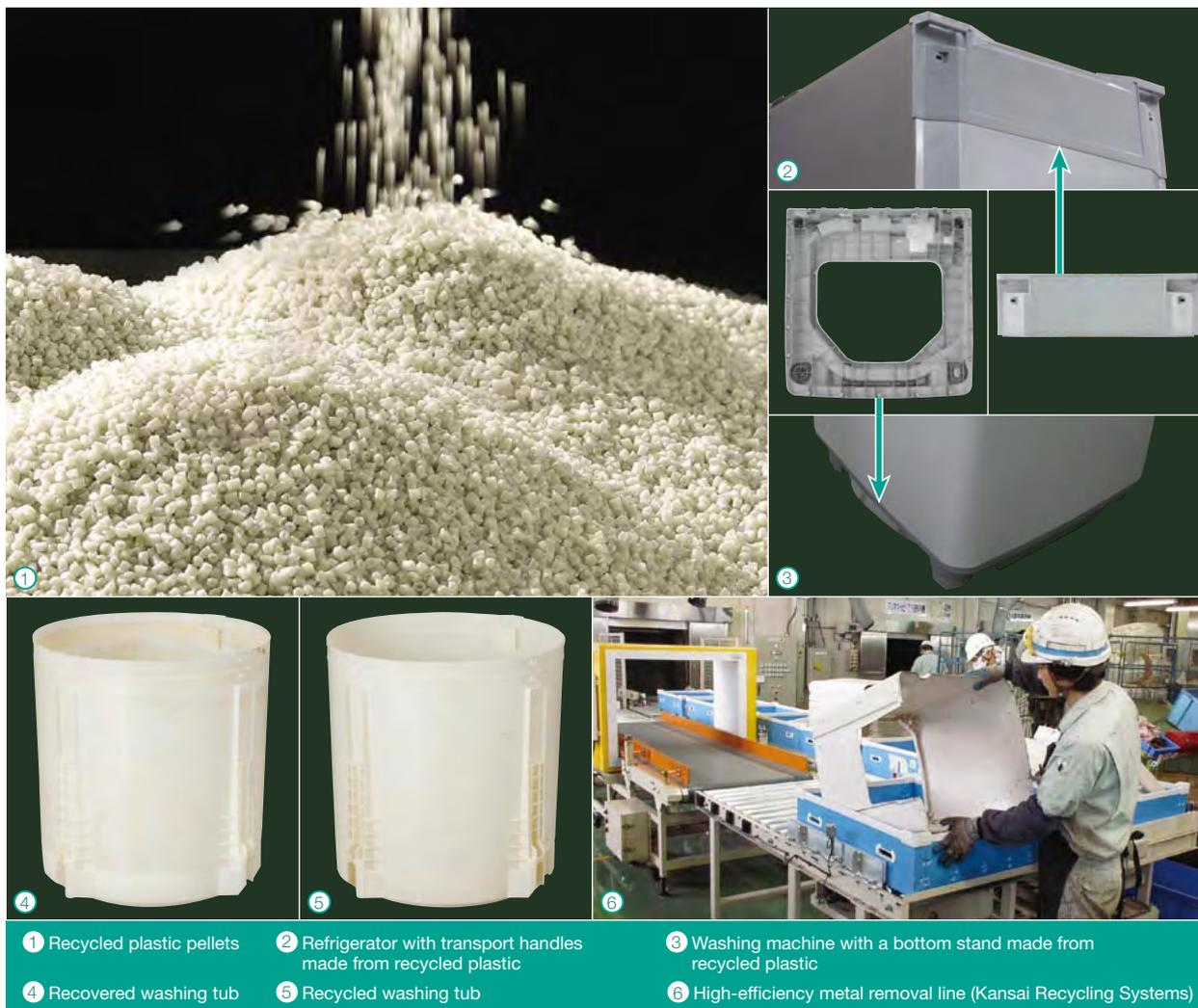
① Recycled plastic pellets    ② Refrigerator with transport handles made from recycled plastic
