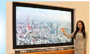
85-inch direct-view LCD compatible with Super Hi-Vision (ultra high definition) (prototype)
