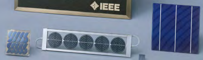
Commemorative plaque from the IEEE (behind) and (from left) two monocrystalline solar modules for lighthouses (installed on the Ogami Island Lighthouse in 1966 and 1978), a monocrystalline solar cell for outer space (installed on the Ume application satellite in 1976), and a residential-use polycrystalline solar cell
