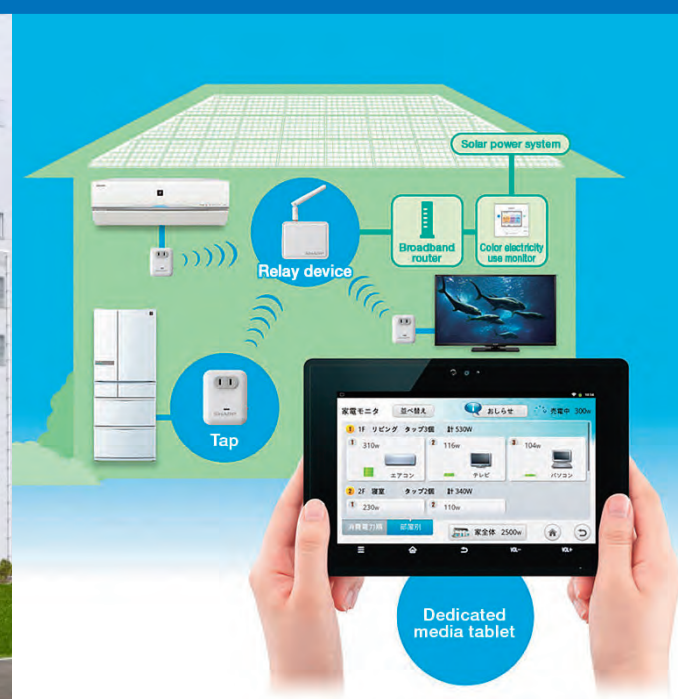
JH-RTP1/JH-RTP2 power consumption visualizing system for Japan (conceptual image). The real-time power consumption of individual home appliances connected to a power-measuring tap can be checked on a dedicated tablet.
