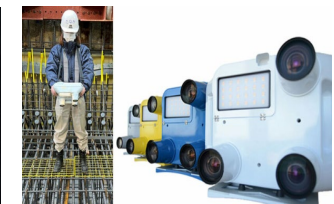
Real-time automatic rebar arrangement inspection system
