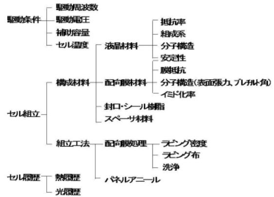
図4 電圧保持率に及ぼす諸要因 Fig. 4 Factors which influence on the voltage holding ratio.
