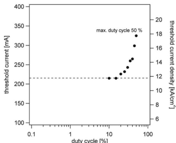
Fig. 7 Threshold current as a function of duty cycle. Measurement on freestanding GaN laser without facet coating at 3.9 °C. The electrical pulse width was kept constant (500 μs).
