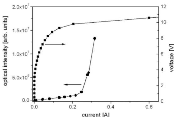
Fig. 6 L-I and V-I characteristics of laser diodes grown by MBE on freestanding GaN substrate.
