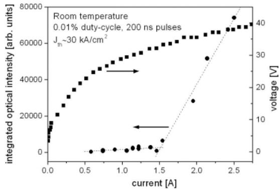
Fig. 3 L-I and V-I characteristics of first MBE-grown laser diodes.
