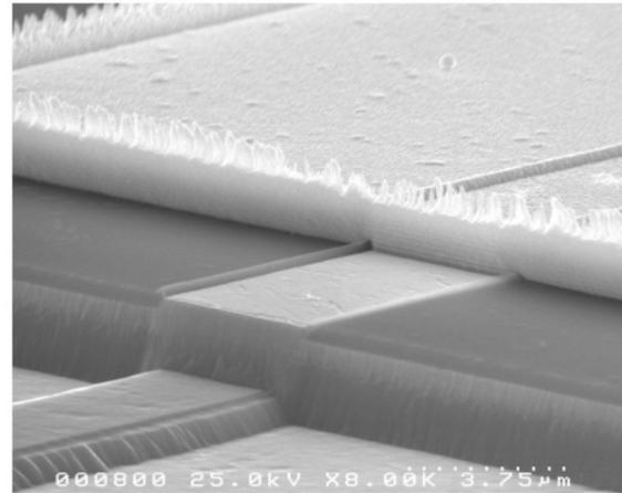
Fig. 2 SEM image of ECR dry-etched laser diode facet.
