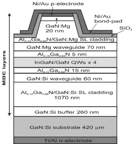
Fig. 1 Structure of the InGaN multiple quantum well (QW) laser diodes as grown on freestanding GaN substrates.
