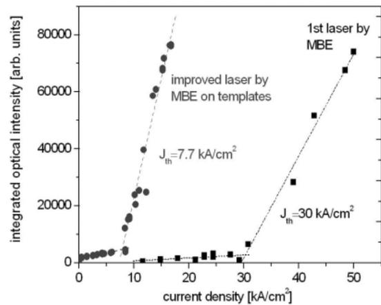
Fig. 5 L-I characteristics of improved laser diode grown by MBE on template substrate, compared to first laser diode on template substrate.
