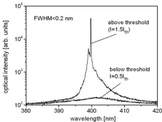
Fig. 4 Emission spectra of typical laser diode below and above threshold.
