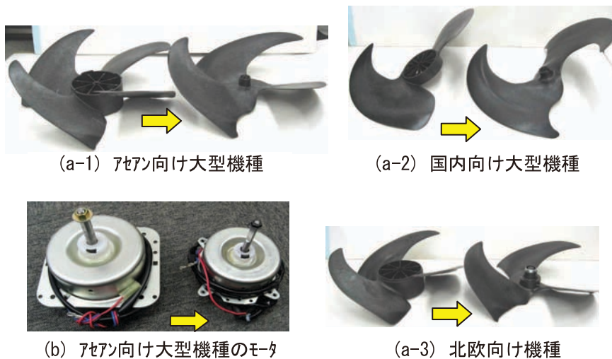
図3 新開発「鳥」ファンの省資源化の効果② (左が従来, 右が新開発) Fig. 3 Effect of saving material by developed fan (2)
