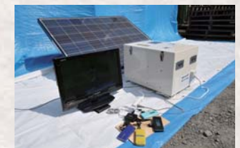
One form of aid was a solar power system for disaster relief that combined solar cells and storage batteries. Produced in collaboration with Shin-Kobe Electric Machinery Co., Ltd., these systems were donated to emergency shelters. The stored power generated from sunlight was used for purposes such as charging mobile phones and watching television.
